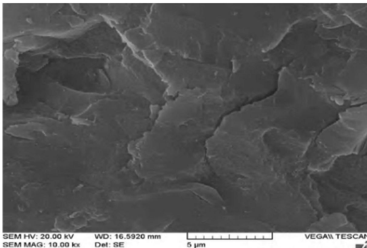
**Figure 2:** The SEM Image of the Activated Charcoal before the Doping
