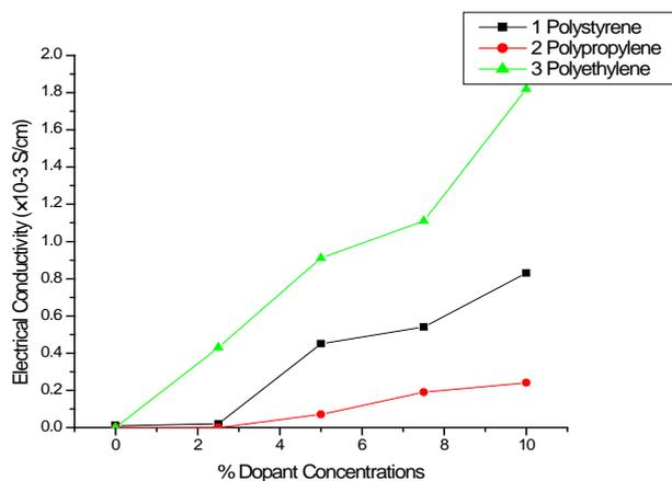
**Figure 4:** Effect of Dopant on Electrical Conductivities of the Polymers.
