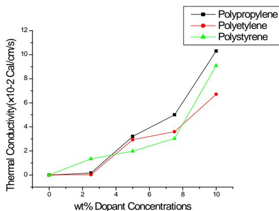
**Figure 5:** Effect of Dopant on Thermal Conductivities of the Polymers.
