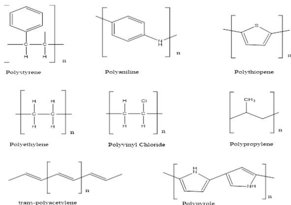
Figure 1: Structures of some conducting polymers.
