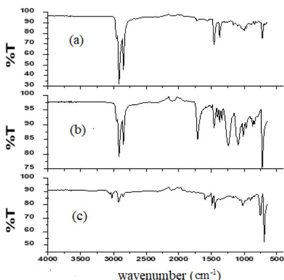
Figure 3: (a, b and c)- The FTIR analysis of the doped PP, PE and PS
